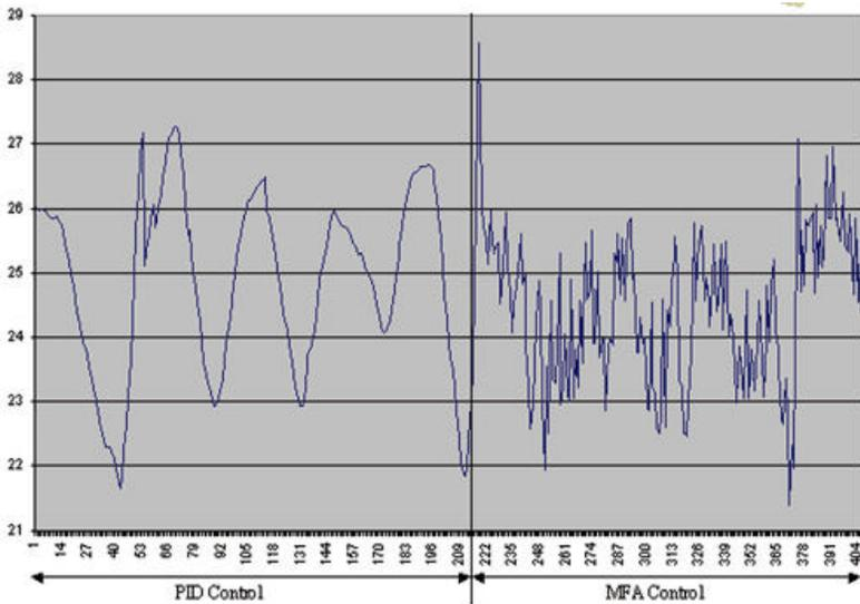
Figure 3 shows the rich liquid reflux flow manipulated by PID and MFA. The MFA output moves with a faster and more intelligent pattern that actually reduces overall variation of the reflux flow. Notice that the frequency is greater in MFA, but the magnitude is similar or perhaps less.
