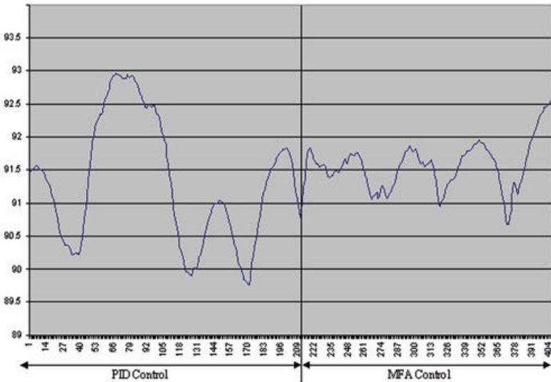
Figure 5 (below) indicates flow of high-value product. It shows a higher and more consistent gas flow with the MFA controller.
